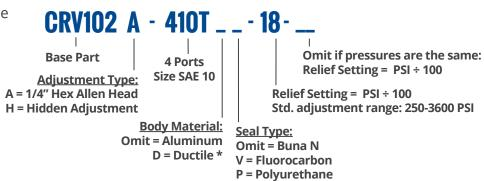
Type "A" adjustment is the standard offering. Hidden adjustment may have a longer lead time. \* Fluorocarbon seals are used when temperatures exceed 212° f (100 ° c).
